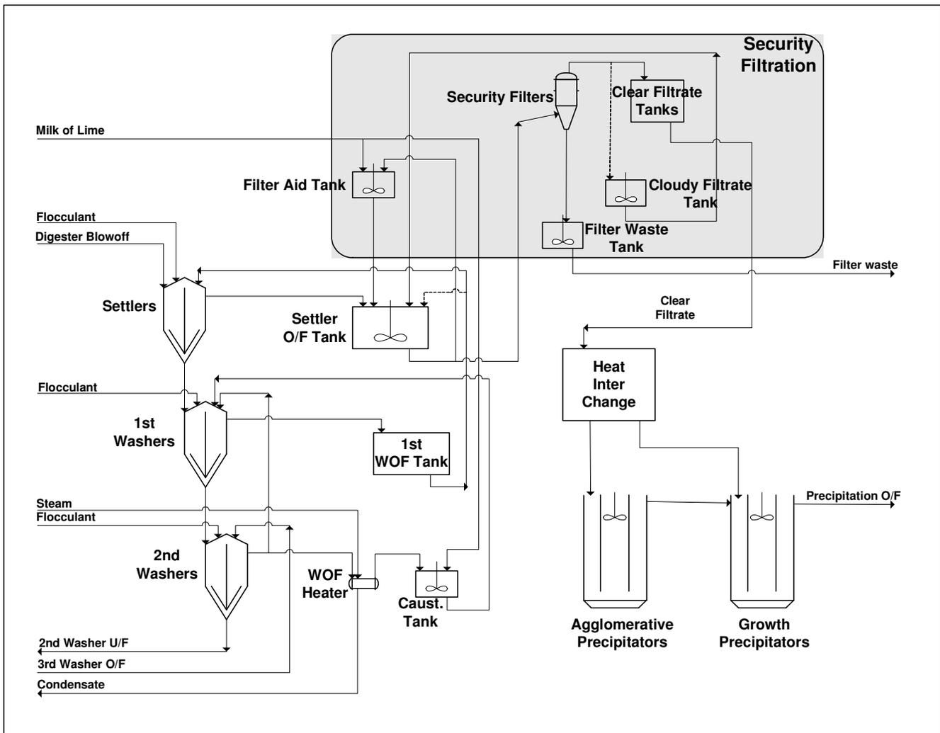
Figure 1 – Security Filtration, Settling & Precipitation
